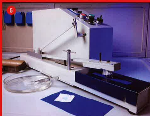
Picture 5: Crock-meter used for the evaluation of brush resistance of treated fabrics
