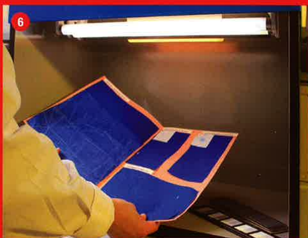
Picture 6: Evaluation of printed fabric samples by light chamber and gray scale
