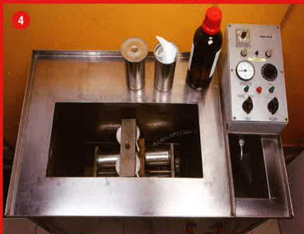
Picture 4: Laboratory machine used for dry washing of fabric samples printed with Crilat 1815
