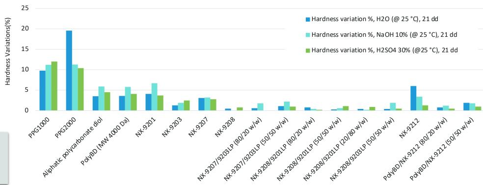
\*NCO: Monomeric MDI, 1,4-BDO extended prepolymers cured at RT for 18 h (T12 and Dabco 8154 have been used as catalysts and BYK 054 as air release additive)
