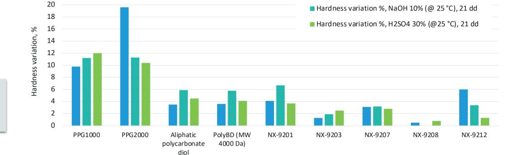
\*NCO: Monomeric MDI, 1,4-BDO extended prepolymers cured at RT for 18 h (T12 and Dabco 8154 have been used as catalysts and BYK 054 as air release additive)
