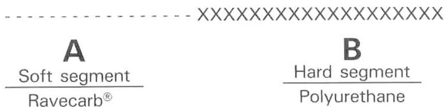
The soft segment is the high molecular weight polyol chain, and the hard segment is the reaction product of the chain extender and the diisocyanate.
