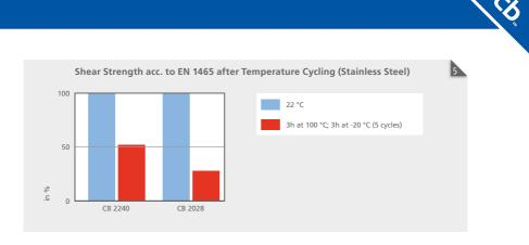
The diagram [Fig. 5] shows a lower decrease of strength after 5 cycles at 100 °C but at -20 °C for 3 hours the partly flexible Cyanoacrylate CB 2240 retains much more of its initial strength, approx 52 percent, whereas the standard ethyl ester based Cyanoacrylate (CB 2028) only retains 28 percent.
