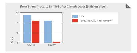
After a climatic load (10 days, 40°C, relative humidity 90%) CB 2240 shows a shear value of around 22 N/mm<sup>2</sup> and conclusively this strength was neither heavily influenced by adhesion or cohesion failure. This is different with standard products. After the climatic tests these standard adhesives did not show sufficient strength anymore. Stainless steel was used as the absence of surface oxidation (corrosion during the test procedure) gives a true reflection of adhesive bond performance.
