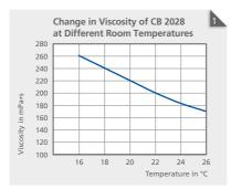
The change in viscosity at different temperatures has to be taken into account [Fig. 1]. The lower the room temperature gets, the higher the viscosity increases and vice versa. This can be of great importance when there are difficult applications. Cyberbond measures the viscosities and setting times at a room temperature of 20°C.
