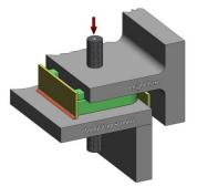
The general rule: form a blocking cavity with no leaks, the foam damming materials and sealant adhesive can be used.
