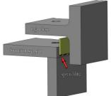
Attach the iron front between the body base and engine base to form the pouring area, the height and distance from the base should be accorded with limits shown. And leak the attachment with the
