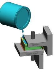
• **Samples:** pour the mixture about 300 g to the appropriate small box, after curing test Barcol hardness.
