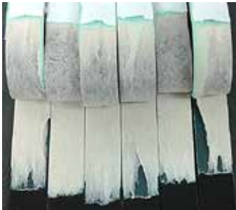
Primed TPO to ABS/PC failure mode at 25°C; TPO failure.
