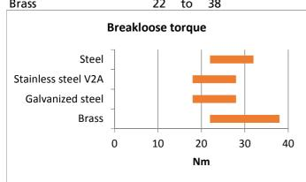
Breakloose torque on M10 bolts and nuts in Nm according to DIN 54454, free swimming without ontorque.
